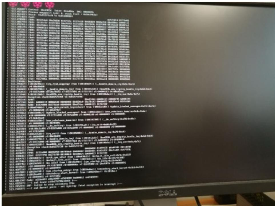
Figure 5: Error message on the screen of a frozen station.
