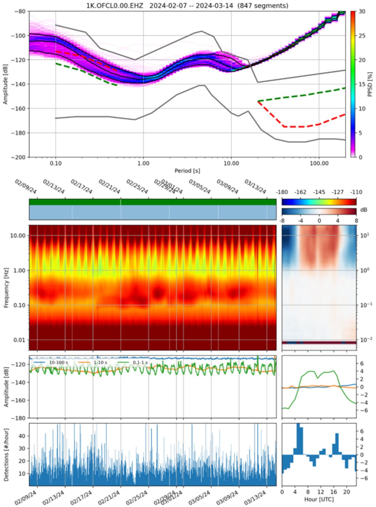
Figure 15: Signal analysis summary sheet of OFCL0 Raspberry Shake stations.
