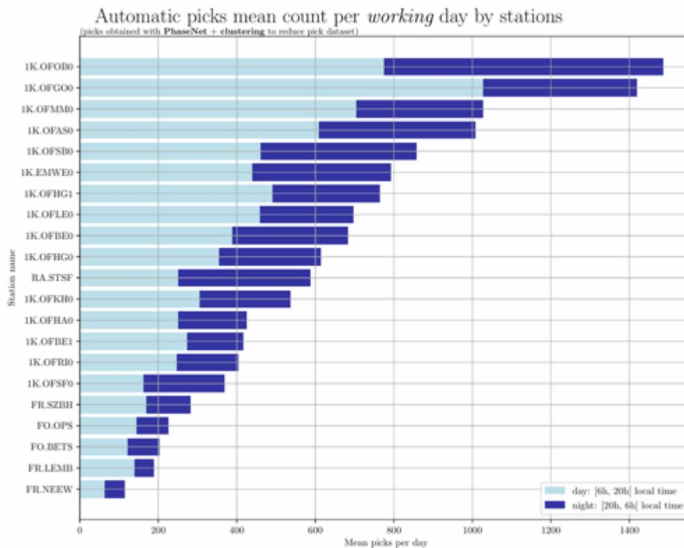
Figure 13: Automatic picks mean count per working day by stations of the Outre-Forêt area. “1K” stations are Raspberry Shake stations, “FR” stations are permanent EPOS-France stations, “FO” stations are geothermal operators stations.
