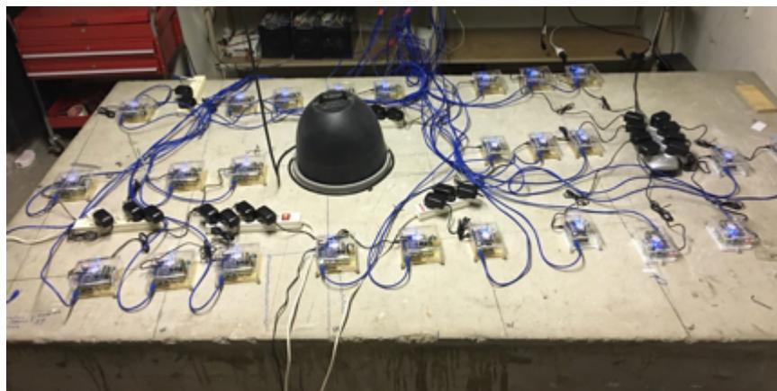
Figure 2: Raspberry Shake stations deployed on the test platform of EOST. The broadband reference station is located at the center of the pillar under the thermal insulating cover.
