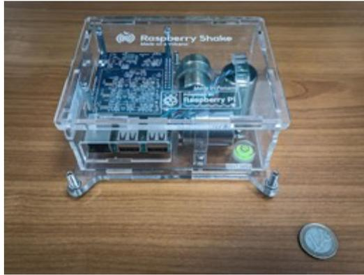
Figure 1: A Raspberry Shake 3D station.
