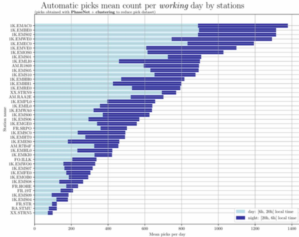
Figure 14: Automatic picks mean count per working day by stations of the Eurometropole of Strasbourg area. “1K” and “AM” stations are Raspberry Shake stations, “FR” stations are permanent EPOS-France stations, “RA” stations are accelerometric stations, “XX” stations are temporary EOST stations, “FO” stations are the geothermal operator’s stations.
