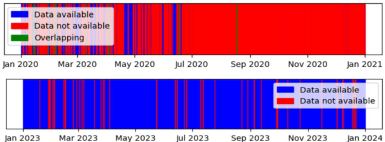
Figure 12: Data availability of station R3374 at BCSF-Rénass before (top) and after (bottom) the change of method of acquisition. Days in red does not mean that no data at all were recovered, but that some gaps are present.
