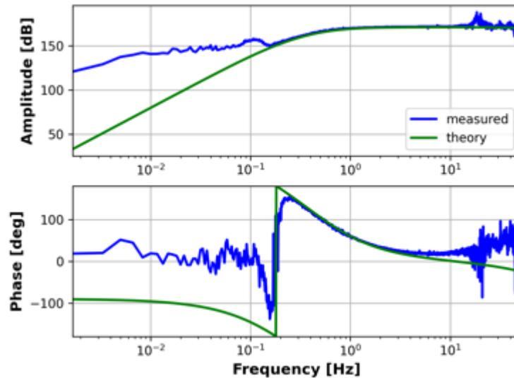
Figure 3: Measured instrumental response of a Raspberry Shake station (blue curve) compared to the theoretical response (green curve).
