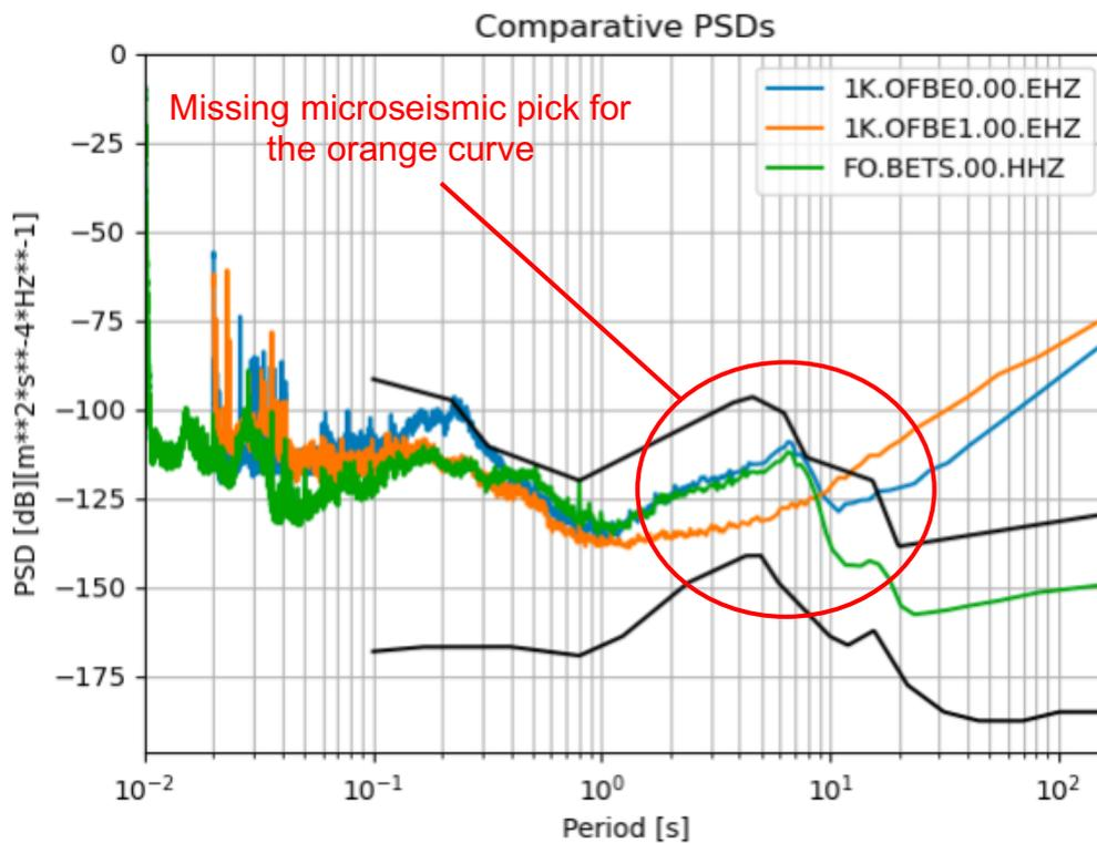
Figure 16: PSD functions of the vertical component of three stations: two Raspberry Shake stations (OFBE0 and OFBE1) and one permanent EPOS-France station (BETS). The three stations are located 1-2 kilometers from each other.
