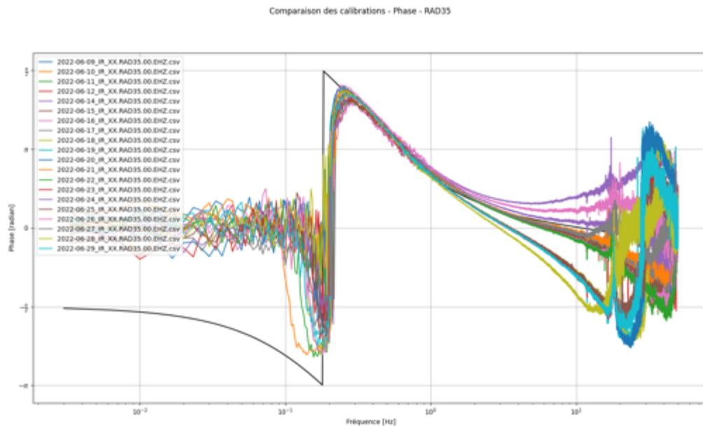
Figure 4: Evolution of the measured instrumental response of a Raspberry Shake station. Each coloured curve represents the measured instrumental response computed for one day. The black curve represents the theoretical instrumental response.
